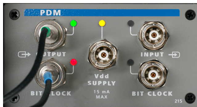
FIGURE 11: APX PDM MODULE, CONNECTING THE APX PDM OUTPUT TO THE PDM INPUT ON A DEVICE
