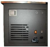
removable panels to allow easy access to the Bath interior. This entry access is shown to the left (closed) and the right (door open).
